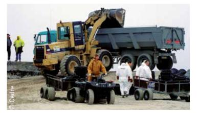
Transfer from beach adapted all-terrain vehicule to truck, for road transportation
