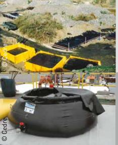
Large open top collapsible container with supporting frame (5 to 140 m<sup>3</sup>)
