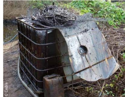
Improvised waste filtration system where recovered oil is passed through a grilled funnel to separate oil and debris
